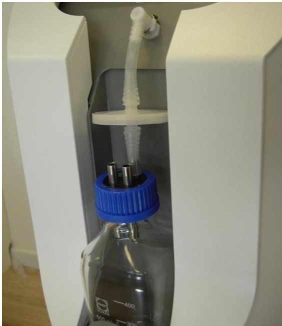
Figure 3-44. Ensemble de filtre installé
